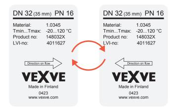
On the valve sticker located on the valve body the flow direction arrow must be changed according to the correct flow direction. New valve stickers can be received from Vexve. vexve.customer@vexve.com
