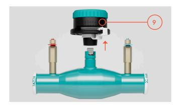
Install the control knop back to the stem. Check that control knop remains in fully open in position 9 and scale remains on the same side of the valve. In the first phase the 2k top of the stem will enter adapter inside of the control knop. After this the anti-rotation part of stem bush will enter control knop. You may need to rotate the whole control knop just a little. Push control knop all the way down on top of the stem and stem bush. Check that control knop is working open/close.
