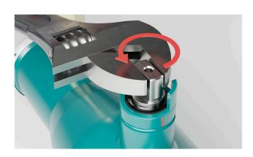
4 Use a wrench to turn the stem 180-degrees. The marking on the top of the 2k is now on the other side of the stem bush.
