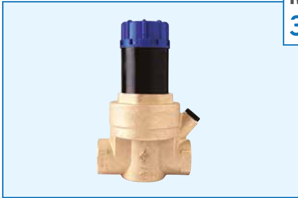
300100* : Pressure reducing and regulating valve with balanced seat, outlet setting from 1.5 to 6 bar. Female/Female threaded connections.
