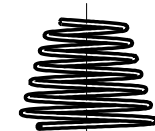
Pos. 9 spring , surface : 6.4 cm 2 , material Aisi 316
