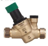
The D04FM is designed to protect household appliances against excessive supply pressures. A small compact valve that will maintain a constant water pressure irrespective of the supply pressure, which is often much higher.
