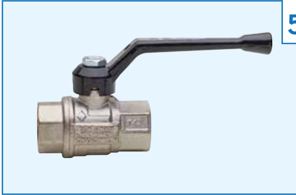
5940* : Degreased full bore ball valve for non-medical oxygen usage, F/F threaded, with aluminium handle.
